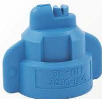
The SoftDrop nozzle is a non-air inducted spray nozzle designed to produce Extremely Coarse and Ultra Coarse droplets for maximum drift control with dicamba, 2,4-D, glyphosate, and other systemic products applied by PWM equipped spray rigs. SoftDrop nozzles are also excellent for liquid fertilizers and mixtures of liquid fertilizers and herbicides.
