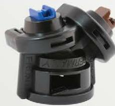
The SprayMax DualFan Nozzle is a non-air injected nozzle that employs conventional flat fan tips in an asymmetric dual cap. The dual tips are oriented 10° forward and 50° rearward to provide a combination of penetration and backside coverage in complex canopies.
